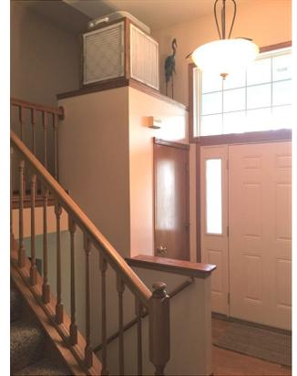
Then there is Made In My Garage...I created a wood frame for the air filter with a fan that is so quiet you can't hear it running. The four MERV 8 filters are more efficient than the single filter in the furnace. The prototype I made using duct tape is in the garage to catch the sawdust made when making the wood frame. Catch 22 but it kept me busy and I enjoyed figuring out the joints and grooves. Yes, I'm easily amused.
